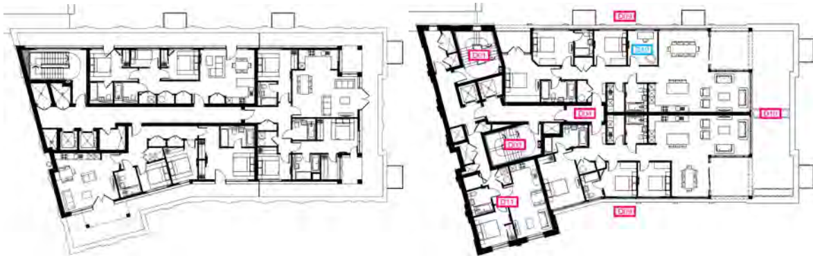
Figure 21 - Approved (left) and marked up (right) proposed eighth floor plans
