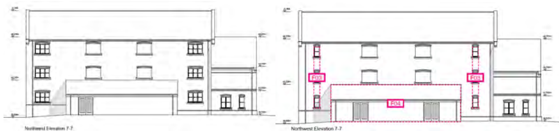
Figure 30 - Approved (left) & marked up (right) proposed west elevation (riverside) plans for Block F&G
